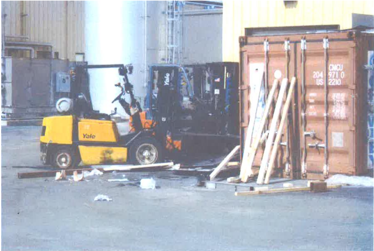
Photo 1 of 1: The employee was struck in the back by the mast of a forklift
