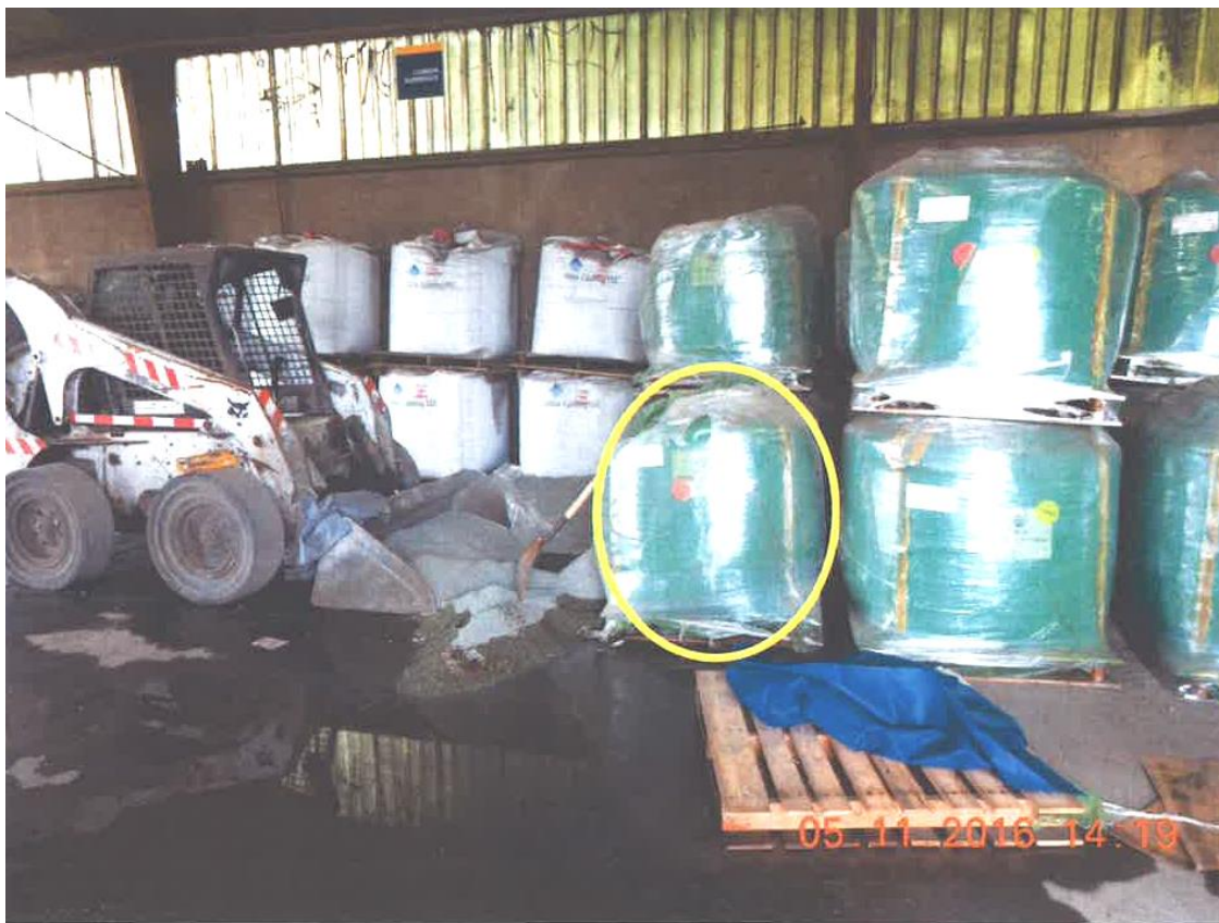
Photo 1 of 1 –The lower tiered super-sack of tap hole sand (yellow circle) where the hole was located.
