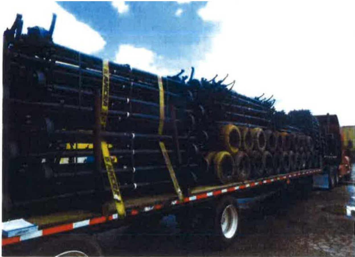
Photo 1 of 1 – Shows a trailer loaded with axels and tires using the same tied down methods as the trailer involved in the incident. The load upright supports shown in the photo were not installed on the trailer involved in the incident.
