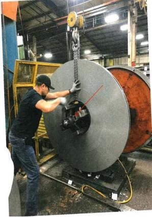
View south to north of coil on uncoiler with installed locking mechanism while still being held by chain strap and Jib Crane.
